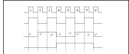
**NOTE:** A mark is allocated for the correct count at each clock pulse e.g. the count at clock pulse 3 should be 011 and at clock pulse 8 the count should be 000.
