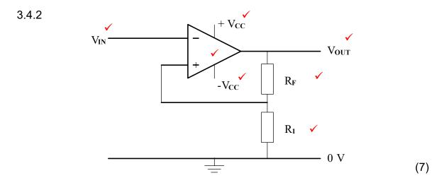
3.5 3.5.1 The gain of the amplifier is determined by the ratio ✓ of the feedback resistance ✓ to the input resistance of each. ✓ (3)
